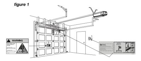
Three warning labels are provided with this opener: attach as indicated in the fig 1 to a clean and suitable surface.
